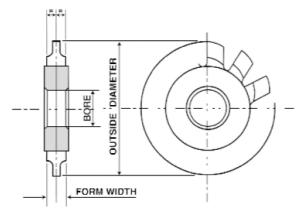
The profiles are made in accordance with BS 978 Part 2, NHS 56702/3 and have square bottoms, also NHS 56704 with round bottoms. These cutters can be sharpened without loss of form. For suitable grinding wheels see right.
